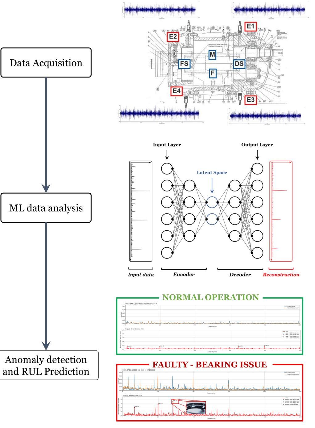
based platform for anomaly detection for industrial and medical infrastructures, tested on CERN's Large Hadron Collider (LHC) cryogenic system helium compressors.
