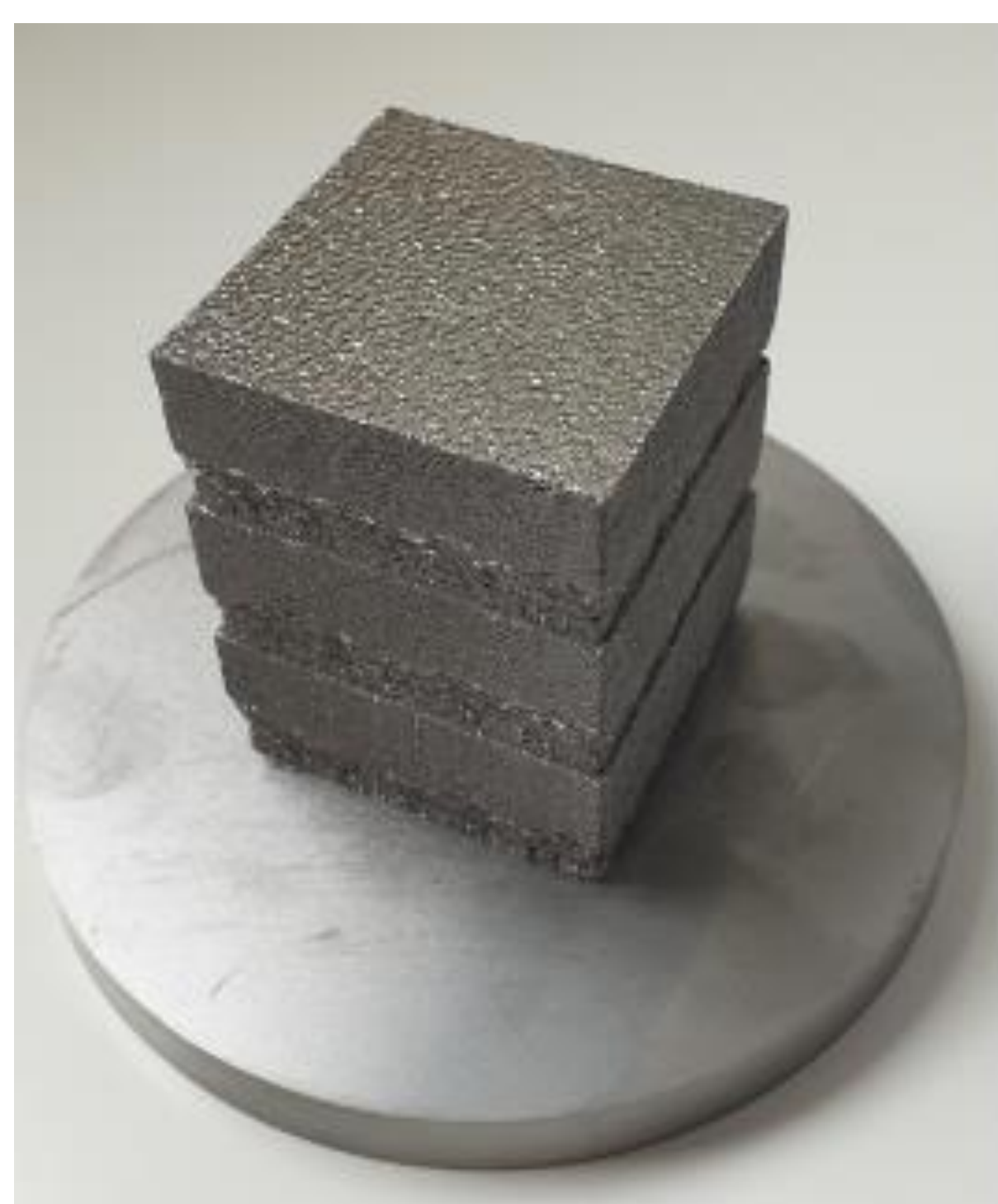
Image 2. Stacked tungsten tiles for fusion energy research
